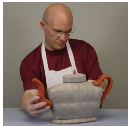
Complex forms can be made from simple templates, and variations on a theme can be explored by altering the templates, the relationship between the templates, or the rib profile used to finish the contours. Other elements, such as handles and spouts can be cast separately and added as needed, but it is a good idea to "fit" the models before making the molds.
