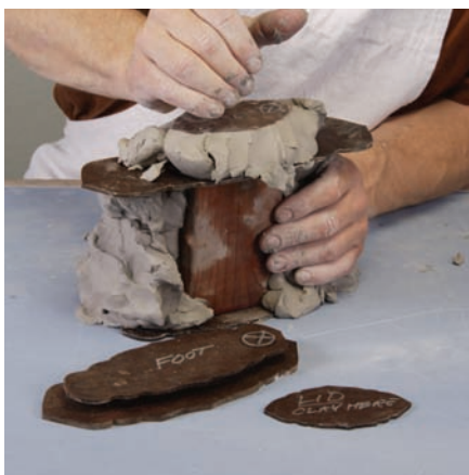
Complex forms can be made from simple templates, and variations on a theme can be explored by altering the templates, the relationship between the templates, or the rib profile used to finish the contours. Other elements, such as handles and spouts can be cast separately and added as needed, but it is a good idea to "fit" the models before making the molds.
