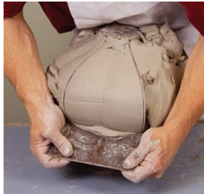
A series of templates that define the various sections of a covered jar are glued together, filled with clay, and scraped to the appropriate profile with a custom-made rib. With this system, the form can be altered in several ways at every step in the design process.
