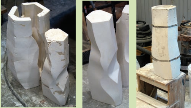
Left: An original plaster form is used to create a waste mold, the working interior surface of which is refined and cast with plaster. Middle: A positive plaster model is cast from the waste mold and is further refined until the final form is determined. Right: From the model, a production mold is made that is used to slip cast porcelain.
